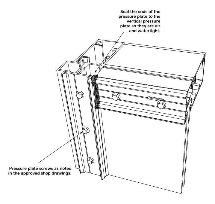
Perimeter Pressure Plate at Jamb
