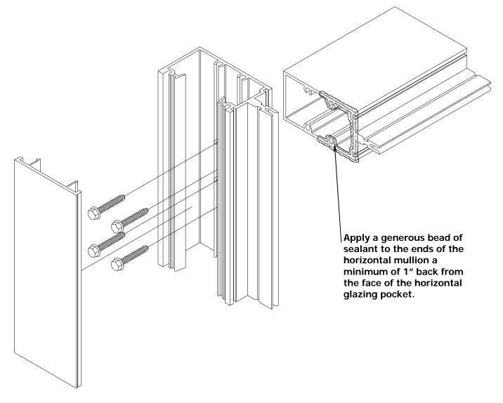
Frame gaskets may be used as an alternate method for frame sealing and are NOT BY EFCO. Use .062 X 3" PVC foam tape with adhesive on one side. Apply the gasket to the end of the horizontals, assemble, and trim the excess gasket from around the horizontal.
