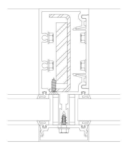
When steel reinforcement is factory installed into mullions, fasteners will be used to prevent damage or slippage of the steel during shipment. This practice is also recommended for the customer on stock length orders.
