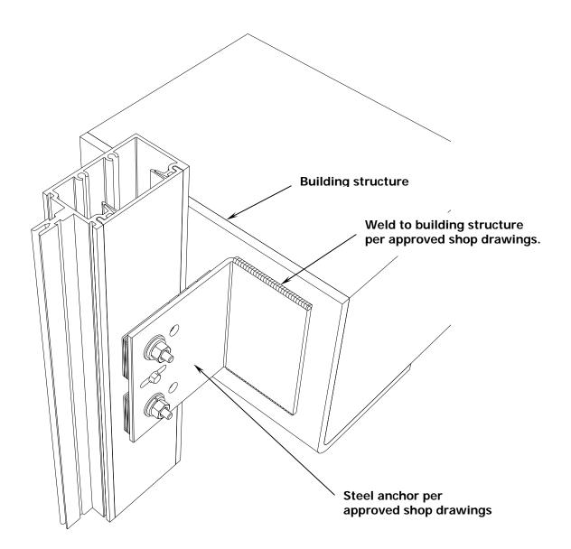
**<u>NOTE:</u>** The elevation of the structure must be within the adjustment limits of the anchoring system. See approved shop drawings for limitations.
