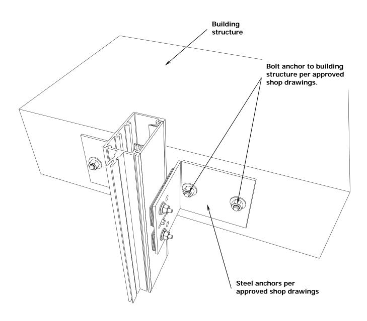
**<u>NOTE</u>**: The elevation of the structure must be within the adjustment limits of the anchoring system. See approved shop drawings for limitations.
