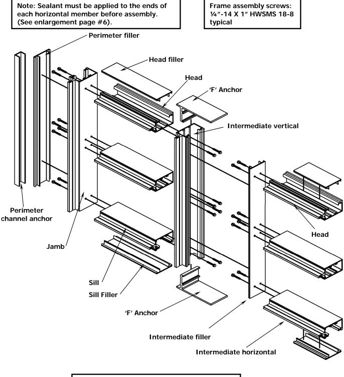
Note: Head and sill fillers above and below 'F' anchors are cut short to avoid anchor bolts.
