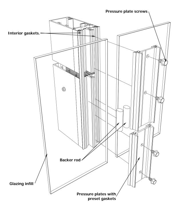
STEP #5 Install and Seal Mullion Splice and Cover
