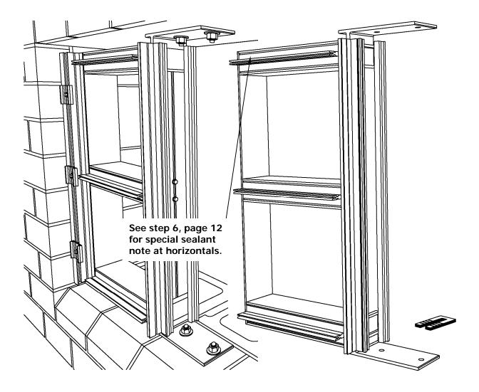
\* NOTE: On long runs, check overall frame dimensions at every fifth opening to avoid dimensional build-up. The commercial cut length tolerance is +/- 1/16". It is critical to check every fifth unit for location relative to established benchmarks.
