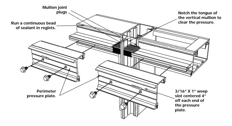
Perimeter Pressure Plate Fabrication at Intermediate Vertical
