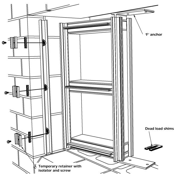
Note: Temporary retainers are available from EFCO by request only and are not included in the cost of the materials for the project. Note: Refer to approved shop drawings for shimming guidelines.
